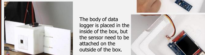
The body of data logger is placed in the inside of the box, but the sensor need to be attached on the outside of the box.
