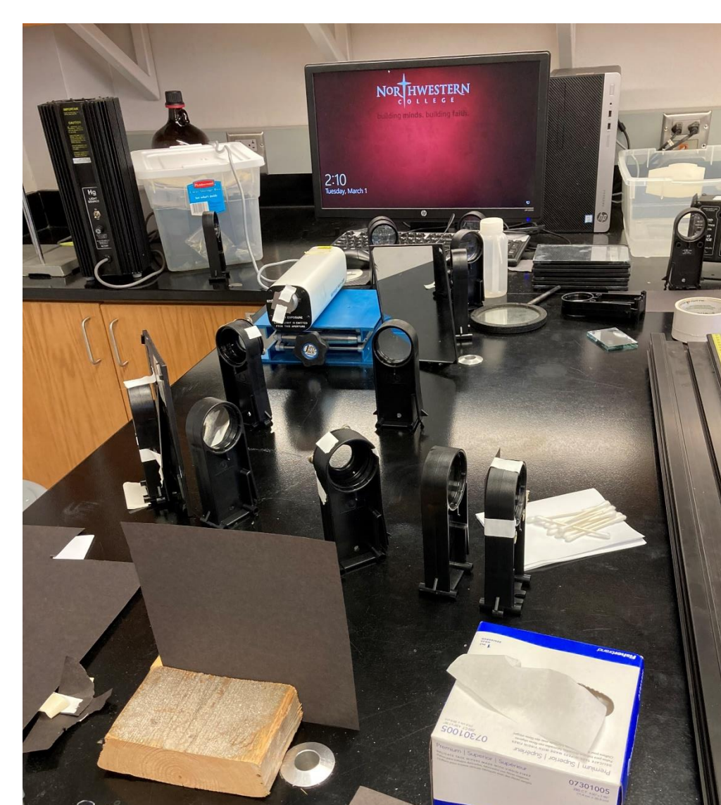
Image 2: our Mach Zehnder interferometer setup in our lab
